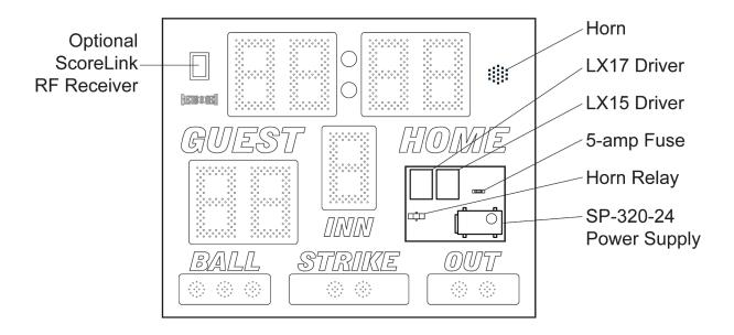
If your scoreboard system includes a ScoreLink wireless data kit, the receiver unit will be located in the upper left corner of the display face. The internal Horn will be mounted in the upper right corner. To access the Horn for service, remove the Period Clock Seconds digit assembly.
